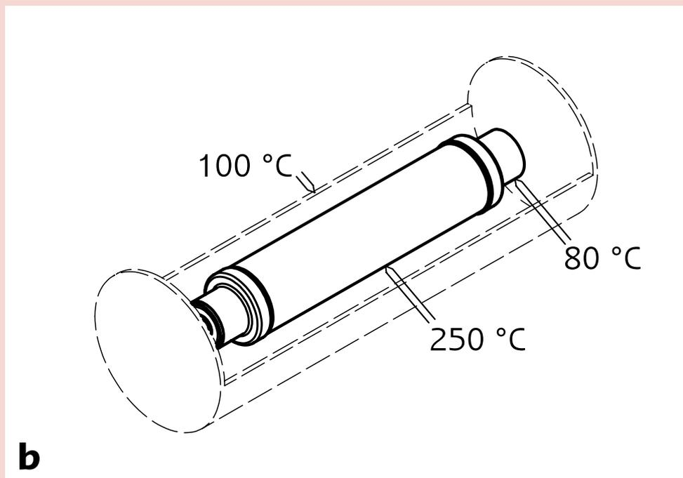
Figure 5: Temperatures at the Fuse Link and the Canister without (a) and with (b) Temperature Limiting Striker Pin
