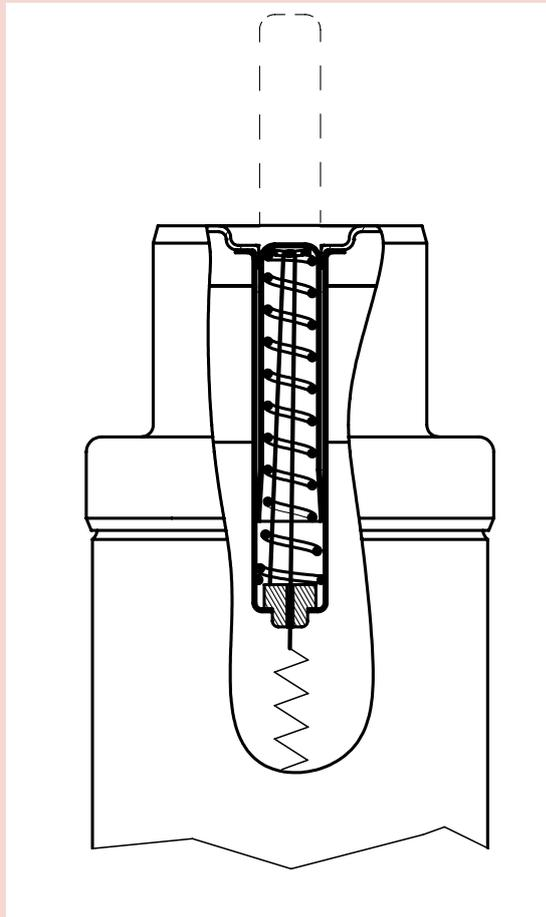
Figure 2: Fuse's Striker Pin
