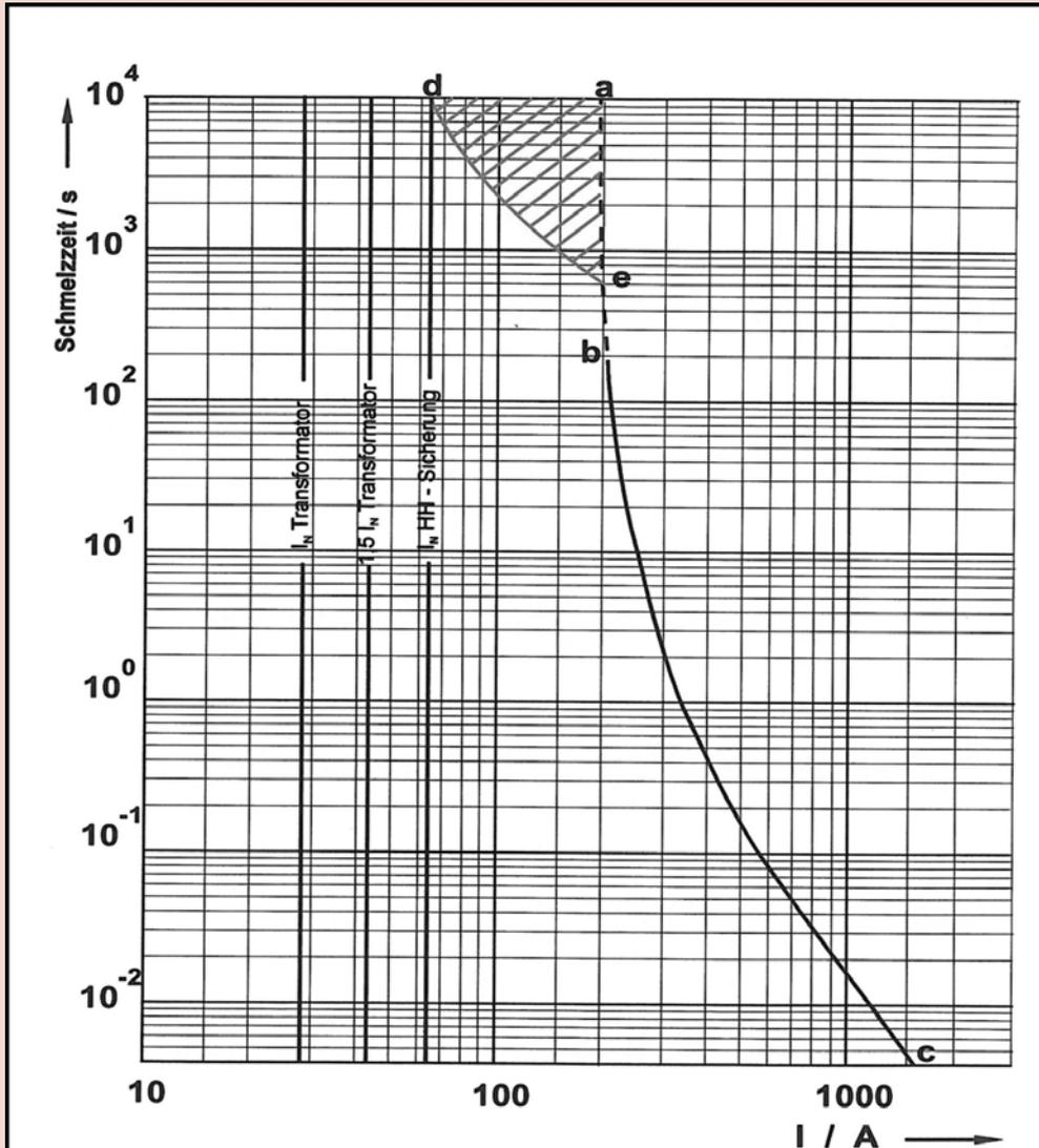
Figure 6: Time-Current Characteristic of a 63 A HV Fuse with a Temperature Limiting Striker Pin in relation to the Operating Currents of a 1 000 kVA Transformer
