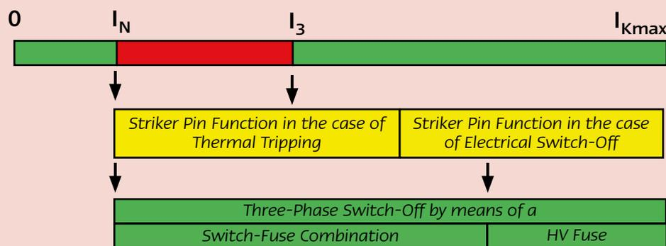
Figure 4: Operating and Breaking Phases of the High-Voltage Fuse
