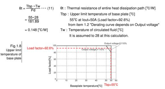
From the thermal resistances  $\theta$ s,  $\theta$ m, and  $\theta$ t obtained in Step 2, calculate the thermal resistance  $\theta$ w required for the water-cooled plate.
