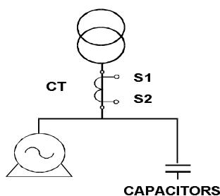
The current transformer , CT, must be located so that it measures the whole load current plus the correction capacitors
