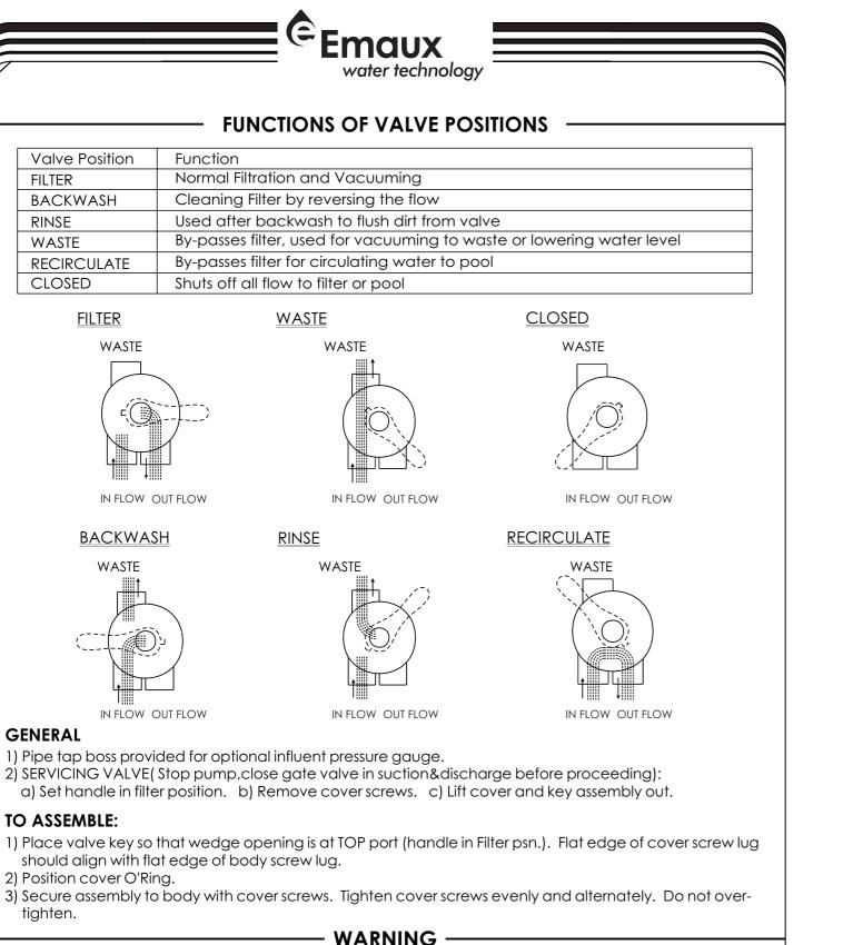
THIS FILTER OPERATES UNDER HIGH PRESSURE. WHEN ANY PART OF THE CIRCULATING SYSTEM (e.g., CLAMP, PUMP, FILTER, VALVES, ETC.) IS SERVICED, AIR CAN ENTER THE SYSTEM AND BECOME PRESSURIZED . PRESSURIZED AIR CAN CAUSE THE LID OR VALVE TO BE BLOWN OFF WHICH CAN RESULT IN SEVERE INJURY, DEATH, OR PROPERTY DAMAGE TURN PUMP OFF BEFORE CHANGING VALVE POSITION.
