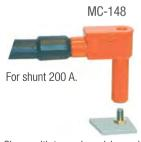
Clamp with tapped revolving rod end M8, 200 A shunt. To be used with an insulating six-sided male hex key 5 mm.
