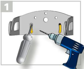
Remove the bracket from the sensor. Drill 2 holes accordingly. Mount the bracket firmly.
