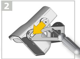
Position the sensor on the bracket and fasten the screws firmly.
