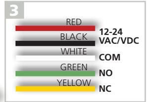
Connect the wires to the door controller. Choose between NO and NC contact.
