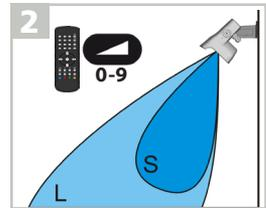
Adjust the field size with the remote control or the push buttons.
