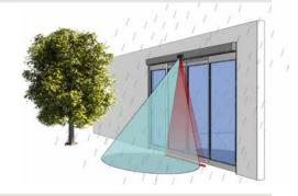
The presetting **SHOPPING STREET**, with a high immunity filter and 2 active infrared curtains is recommended for sensors that are installed in a shopping street with a lot of pedestrians. The door opens only when a pedestrian is detected in both the radar field and the infrared field. This way, unwanted detections are very rare.
