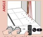
Activate the visible\* spots to verify the position of the IR-curtain.
