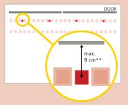
\* Visibility depends on external conditions. When spots are not visible, use the Spotfinder to locate the curtains. \*\* The distance between the inner curtain of the inside door sensor and the inner curtain of the outside door sensor should always be smaller than 20 cm. The distance to the door leaf depends therefore on the thickness of the door leaf.
