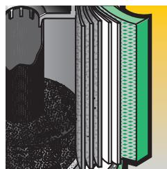
**OIL VAPOR REMOVAL FILTER**for removal of oil and hydrocarbon vapors normally adsorbable by activated carbon; removes solid particles to 0.01 micron (0.003 ppm w/w maximum remaining oil content)<sup>2</sup>
