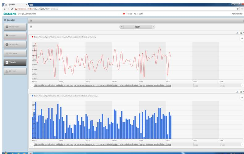
*Checking the dynamic response of the plant using a touch panel or a Web client*
