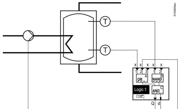
The measured value at input 1, OR Logic A, gives the switch on command for storage tank charging.
