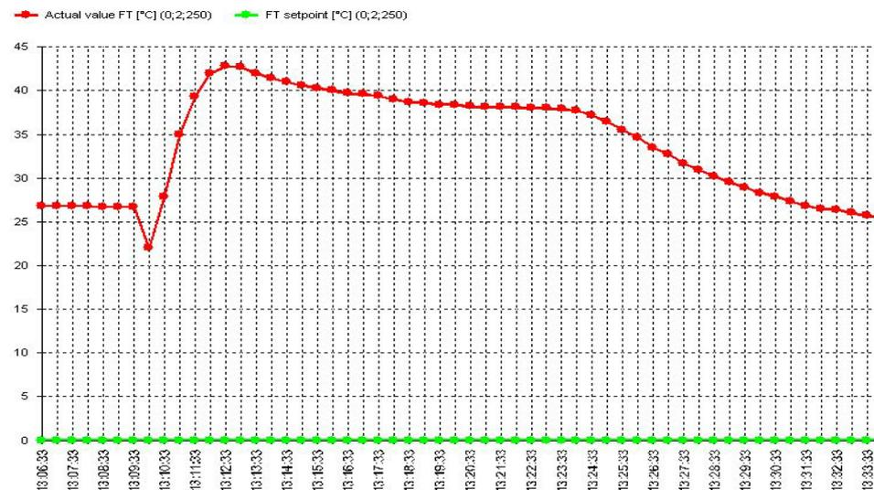
The trend graphs show the data point values according to the sampling interval (graph above is based on a sampling interval of 1 minute).
