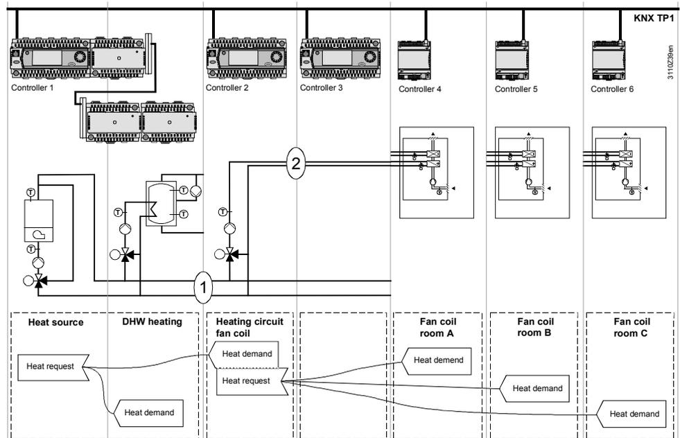
Together with the Synco controllers, which ensure the production and distribution of heat/cooling energy, the room controllers make certain the required room temperature is reached at the right time.
