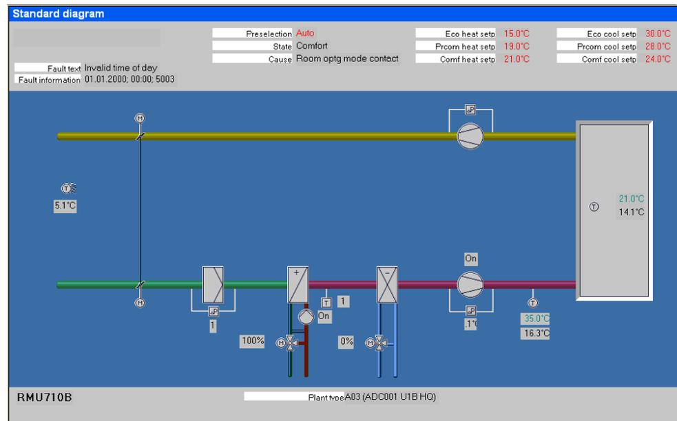
Standard plant diagrams can be copied and then adapted. This means that a user-defined plant diagram can be created from a standard plant diagram.
