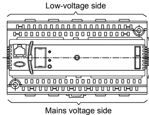
Connection terminals carrying protective extra low-voltage (e.g. for sensors and KNX bus) are located on the low-voltage side (top of the housing).
