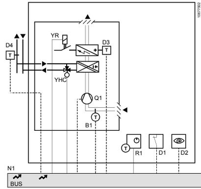
FNC03 2-pipe system with changeover and electric reheater
