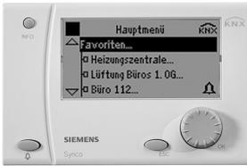
The RMZ792 operator unit of the B-series (see Data Sheet N3113) is used to control from a remote location Synco 700 controls, central communication units, RX.. room controllers and RD.. room thermostats in a KNX network. Basic design and dimensions are identical to the RMZ791 operator unit.
