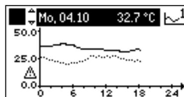
24-hour log showing primary trend (solid line) and reference trend of an additional channel (dotted line)
