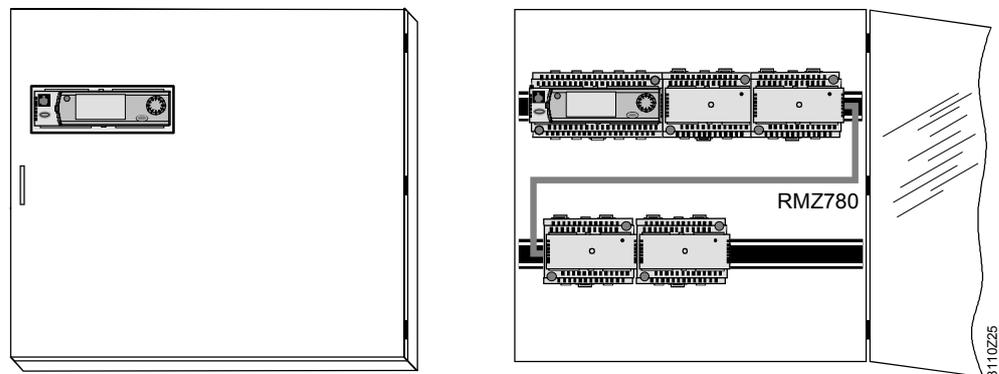
Note: In place of the attachable RMZ790 operator unit it is also possible to use the handheld operator unit RMZ791.
