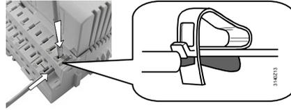
2 Push on the spring cage terminal with a screwdriver and, at the same time, insert the wire
