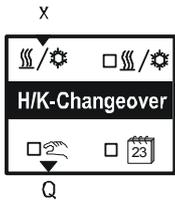
Operating mode changeover from heating to cooling, or vice versa, takes place via function block "H/C changeover".
