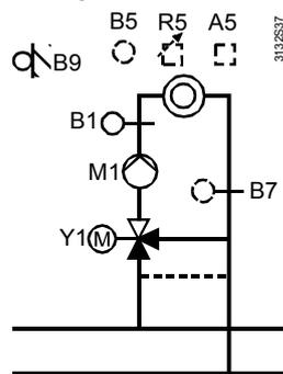
Weather-compensated pump heating circuit
