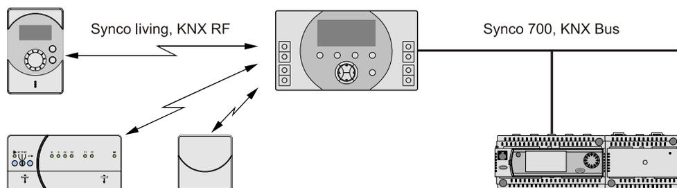
The central apartment unit forms the link between Synco living and Synco 700 controls on the KNX bus.
