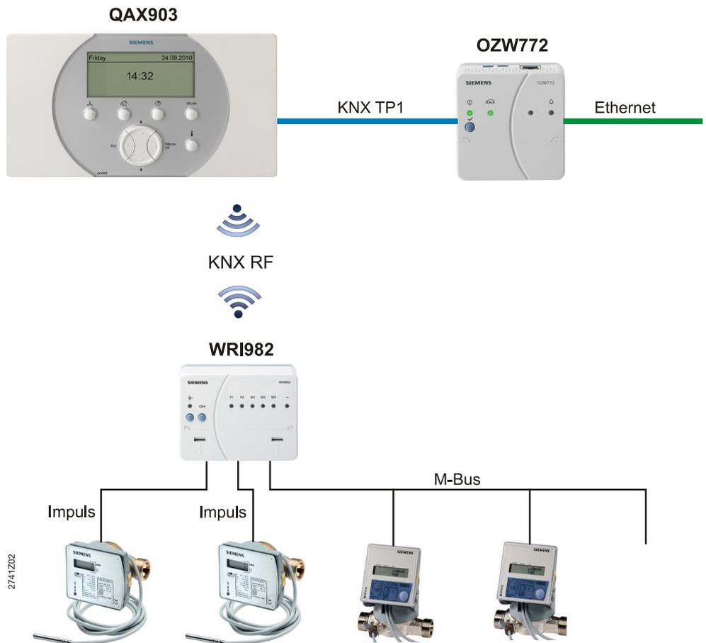
Integrating the consumption data interface WRI982 allows for displaying energy consumption on the central apartment unit and sending it to a service provider via web server OZW772.
