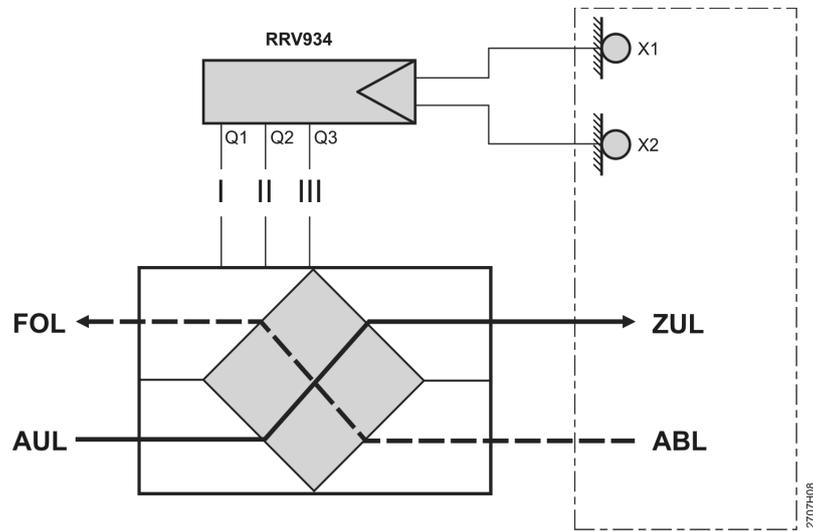
Q1 - Q3 3-stage step selector of ventilation plant
