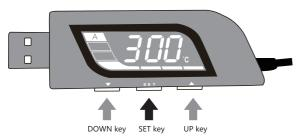
1 Enable to change the storage temperature with SET key; short press the SET key.
