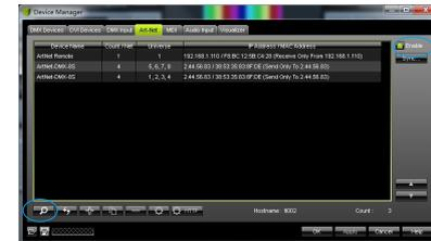
7. Click the tab of "DMX devices", set port status to "ON" if connected successfully. Now, you can use computer to control lamps via ArtNet-DMX-8.
