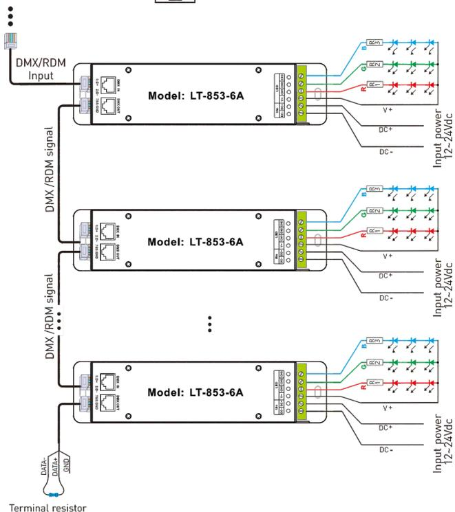
\* If the recoil effect occurs because of longer signal line or bad line quality, please try to connect 0.25W 90-120Ω terminal resistor at the end of each line.
