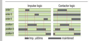
To enable control, close contact 312 with 317. To force the product to 0 position/OFF bridge the contact 313 with 317. For contactor logic bridge contact 316 with 317. To operate: close the contact corresponding to the desired position.
