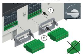
2 Connect the product with a cable of ATyS Voltage section of 1,5 to 2,5 mm<sup>2</sup>. Sensing and Power supply Screw M3 - Tightening torque: min.: 0.5 Nm - max.: 0.6 Nm min.: 4.43 Ibin - max.: 5.31 Ibin Kit excludes the need for fuses F1 & F2. 63A64A24 14 04 13
