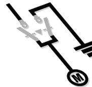
Safely isolating a load from the supply whilst earthing equipment such as motors or electrical lines. This enables work to be carried out downstream of the transfer switch in total safety.
