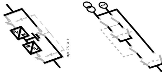
Isolation of the a transfer switch, a UPS or other equipment for scheduled maintenance or tests. This is done by safely disconnecting upstream and downstream circuits, whilst continuing to supply the load via a parallel circuit referred to as a Bypass circuit.
