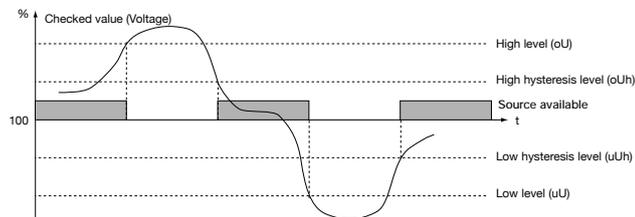
High and low thresholds with time delay define the stable power supply range of the load. High and low hysteresis levels are generally associated with a new stable condition.
