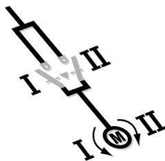
Inversion between two out of three phases supplying a motor in order to modify the direction of rotation. This application requires a delay in the off position to prevent damage to the equipment.
