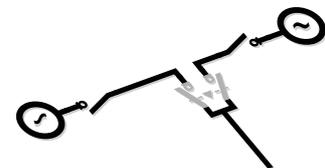
'Normal/emergency' applications are dedicated to safety installations. They ensure continuity in the supply to the loads and facilitate evacuation of the building for security matters. Typical safety equipment include lighting, alarm systems (fire..), smoke extraction systems, fire pumps, air compressors, sprinkler systems, lifts, ...
