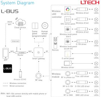
Wifi-108 can be controlled by remote or local LAN, and supports ECHO amazon voice speakers. The E series panel does not support advanced mode when work with WiFi-108.
