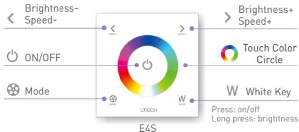
\* When blue status light of key is on, long press to turn on/off buzzer. When white status light of key is on, long press to match code.
