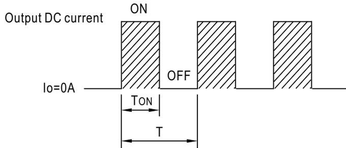
$$\text{Duty cycle(\%)} = \frac{T_{ON}}{T} \times 100\%$$
