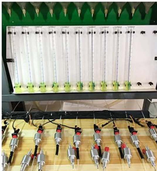
Oil pump test
