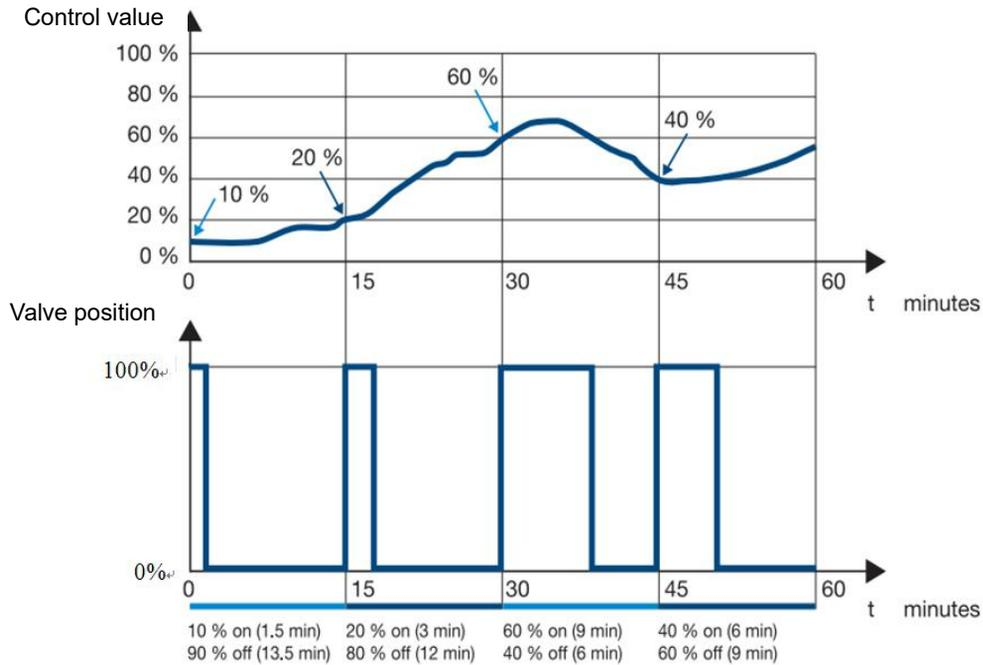
This control mode enables relatively accurate temperature control without temperature overshoot. Simple, low-cost control valves can be used. For example, it can be used in conjunction with an electric valve actuator. The switching frequency of the control valve is relatively high.
