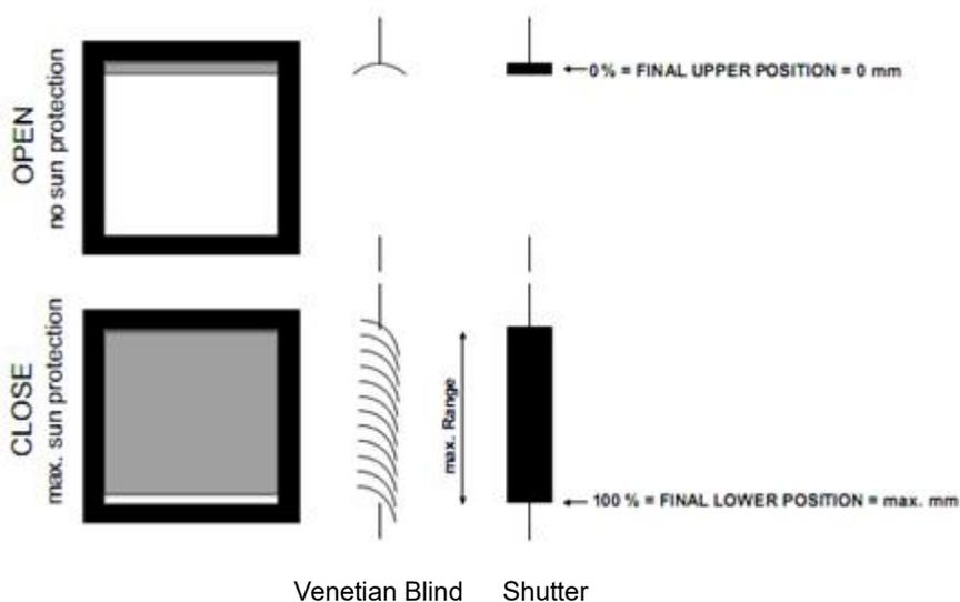
The "Shutter" working mode is not introduced here. The function can refer to the "Venetian Blind" working mode (except for the louver adjustment function).
