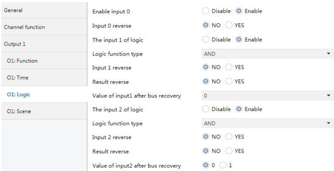
Fig. 4.8 Parameter window "Ox: Logic"
