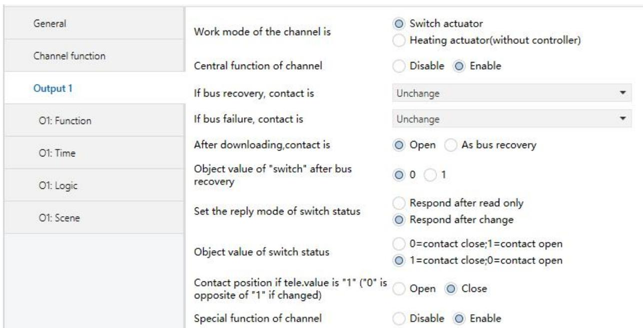
Fig. 4.3 Parameter window “Output X: Switch actuator”
