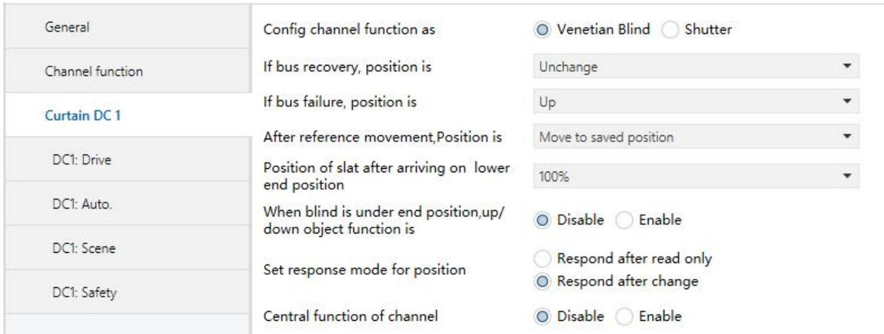
Fig. 4.19 Parameter window "Curtain DC X"
