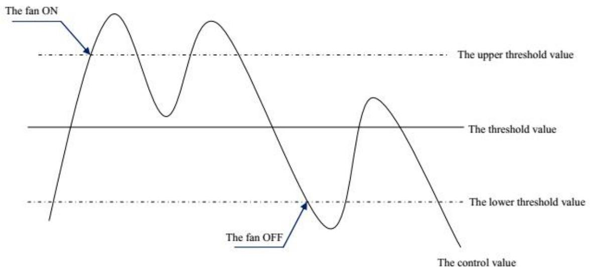
The following parameters in this subsection are descriptions of fan speed control values.
