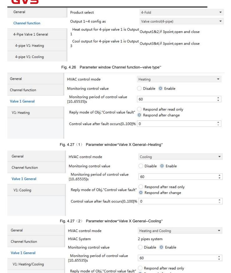
Fig. 4.27 (3) Parameter window"Valve X General--Heating and Cooling (2-pipes)"
