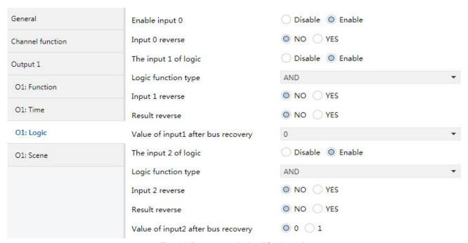
Fig. 4.8 Parameter window "Ox: Logic"
