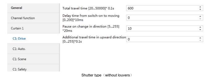
Fig. 4.15 Parameter window "Cx: Drive"
