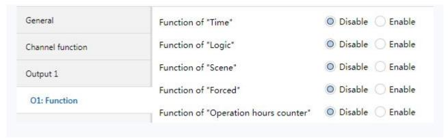
Fig. 4.4 Special function enable setting interface "Ox: Function"
