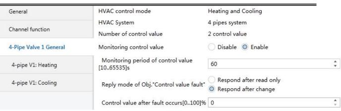
Fig. 4.28 Parameter window"4-Pipe Valve X General--Heating and Cooling (4-pipes)"
