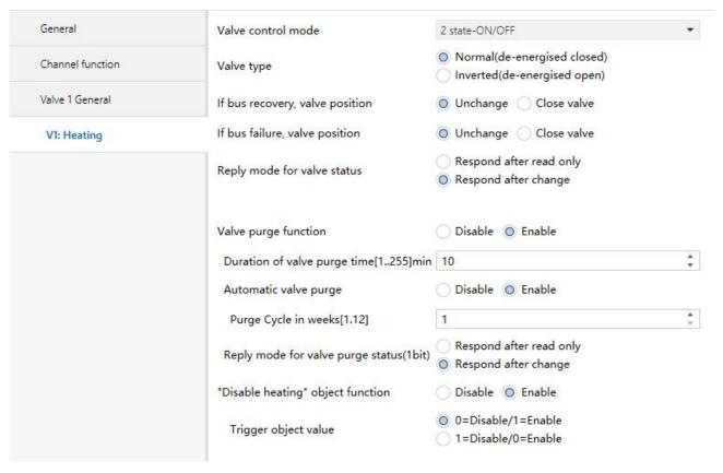
Fig. 4.31 Parameter window "2 state-ON/OFF"
