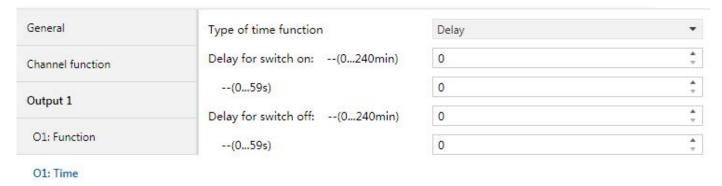
Fig. 4.5 Parameter window "Ox: Time-Delay"
