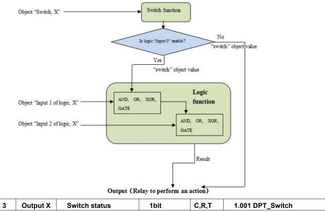
The value of this communication object (Specifically set in the parameter "Object value of switch status:" in Figure 4.3 "Output X") Can directly indicate the status of the relay contacts.
