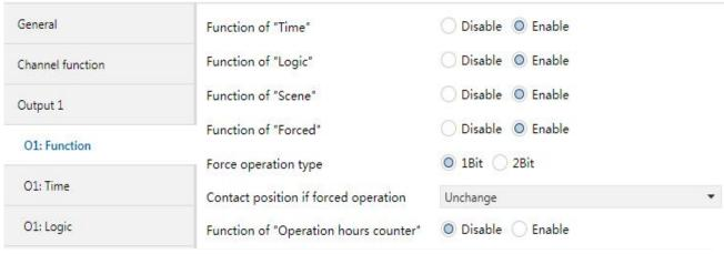
Fig. 4.10 Parameter window "Ox: Forced"
