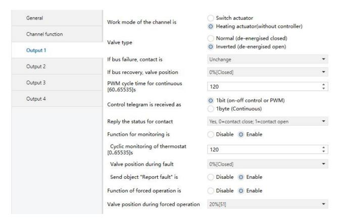
Fig. 4.12 Parameter window"Output X: Heating actuator(without controller)\_1bit (on-off control or PWM)"
