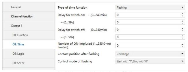
Fig. 4.6 Parameter window "Ox: Time-Flashing"
