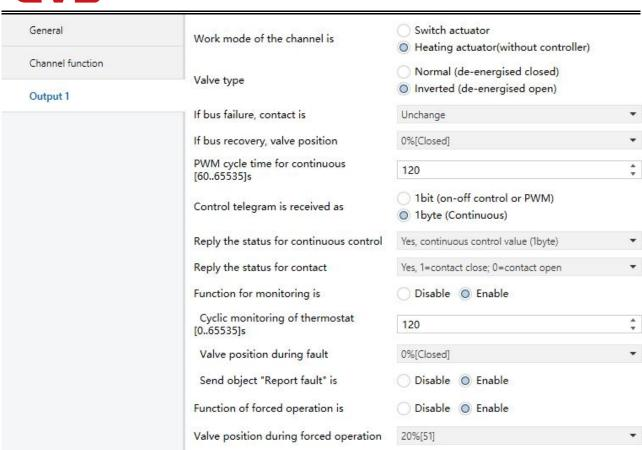
Fig. 4.13 Parameter window "Output X: Heating actuator(without controller)\_1byte(Continuous)"
