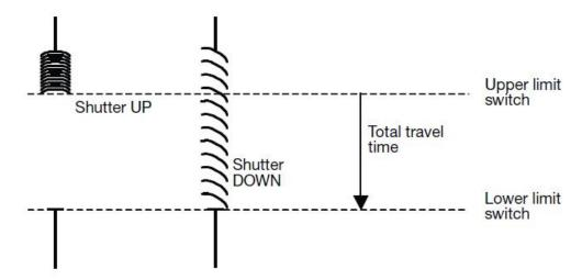
Note: The current position of the Shutter during operation can also be determined with the help of the total move time. It is therefore important to measure and set the total move time as accurately as possible, particularly if the functions "Move to position via a 1 byte value" and "Status response" are used. Only then is it possible to calculate the current position of the Shutter precisely.
