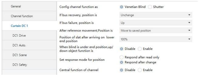
Fig. 4.19 Parameter window "Curtain DC X"
