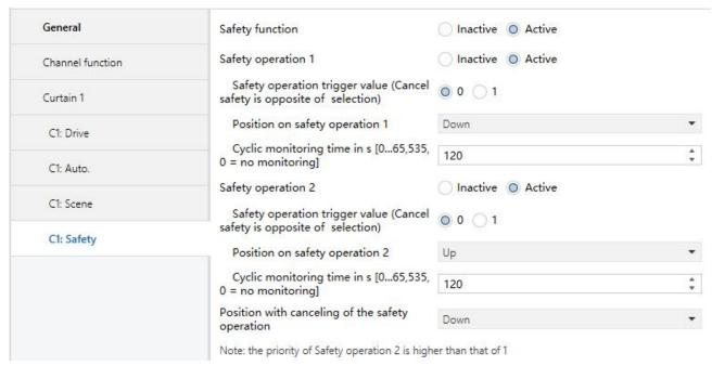
Fig. 4.18 Parameter window "Cx: Safety"
