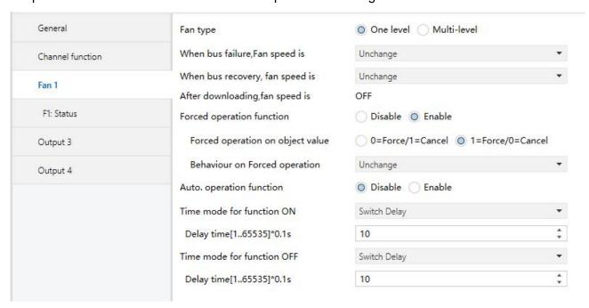
Fig. 4.20 Parameter window "Fan type -- One level"
