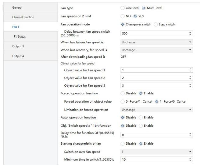
Fig. 4.23 Parameter window "Fan type - Multi-level"
