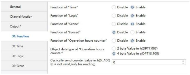
Fig. 4.11 Parameter window "Ox: Operation hours counter"
