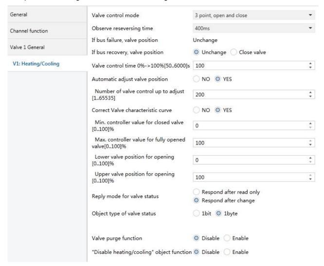
Fig. 4.33 Parameter window "3 point, open and close"
