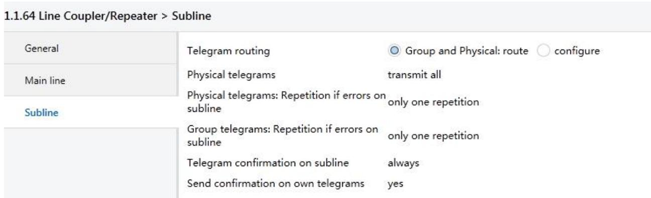
Fig.5.6 Parameter window “Sub line”
