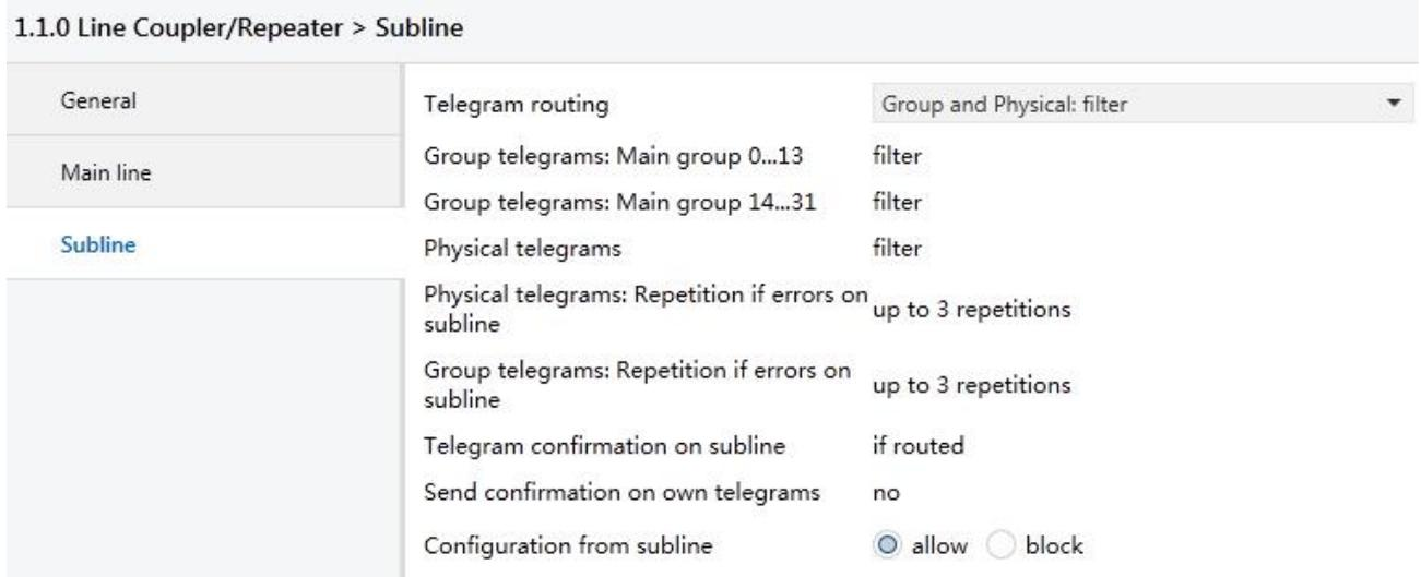
Fig.5.3 Parameter window “Sub line”
