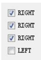
1. The check box is used to select the channel, if select, the channel is for right, if not select, for left. The channel select need be matched with the channel setting of the RF KNX transceiver.
