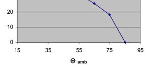
Max. allowable current (rms) at specific ambient Temp.
