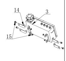
3. Please install the junction box vertically onto the light bracket, make sure the aviation plug facing outward.
