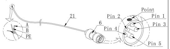
sure no short circuit of Pin 3, 4 and 5 in five core aviation plug (small). Make sure single core's color of 'A', 'B' and 'PE' on both ends of the wire are the same.
