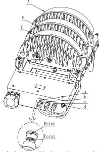
Notice: The white dots on male and female terminals are positioning point, can only be plugged in when they are matched. Tightly screw the nut on the aviation plug to avoid poor wire contact.
