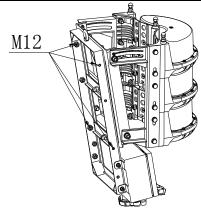
6. After fixing the light head, put the Gradienter (no. 11) on the top of the light case to make sure the light is fixed horizontally. If the light is not fixed horizontally, please adjust according to step 7(below).
