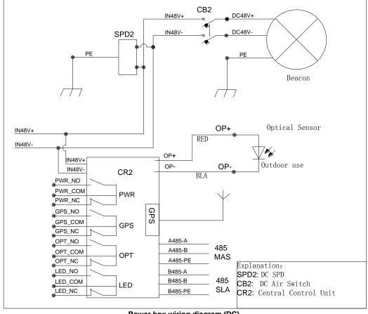
Power box wiring diagram (DC)
