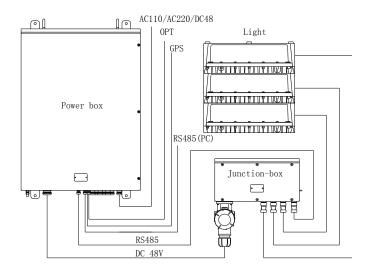
DC power supply wire between the power box output and the junction box. Wire specification as below chart:
