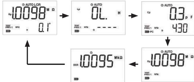
In the manual LCR mode, the meter automatically selects the series/parallel mode depending on the total equivalent impedance measured similarly to the Auto LCR mode. (Refer to 4-7)
