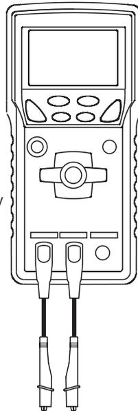
4. Connect the test leads to make a short circuit.
