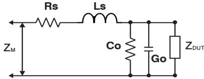
$Z_M$  is defined as total impedance measured to a DUT by a test fixture which has some parasitic impedance.
