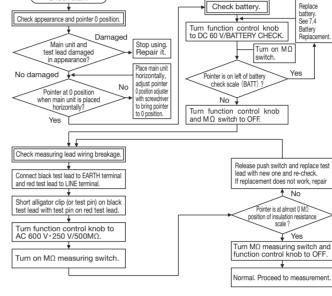
battery. A consumed battery will cause not only measurement errors but danger due to erroneous measurement.
