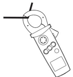
Force applied to the tip of clamp sensor.
