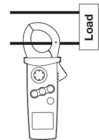
Clamping single conductor on the center of clamp sensor.
