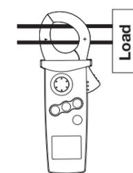
Clamping multiple conductors.
