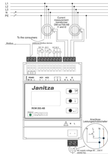
Fig. 4: Circuit diagram of the RCM 202-AB
