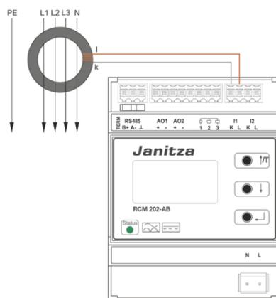
Fig. 3: Simplified presentation of residual current measurement
