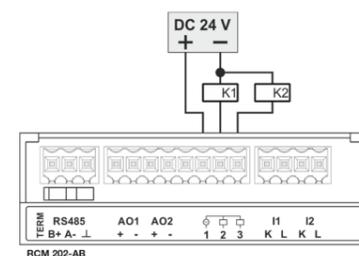
Fig. 5: Connection of two relays to the digital outputs
