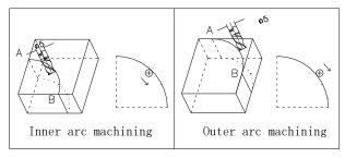
Set the tool radius according to the actual milling cutter when process XY plane.
