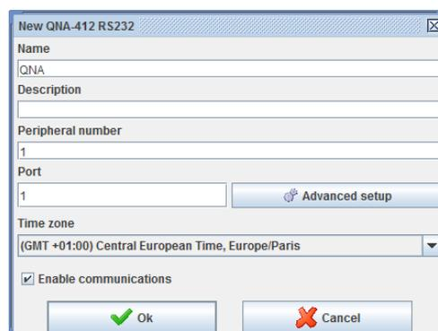
Figure 86:Dialogue box for configuration of QNA412 RS232 communications
