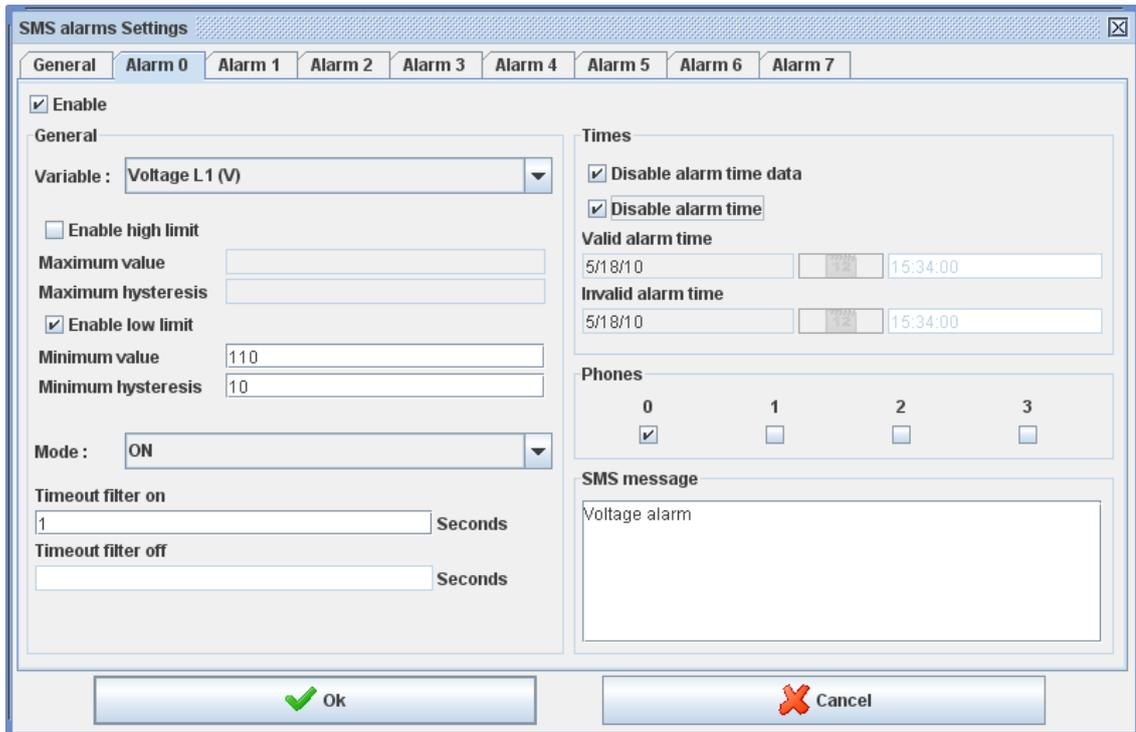
Figure 101: Dialogue box for alarm setup enabling the first alarm
