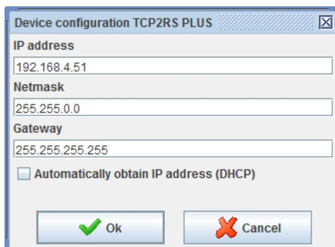
Figure 47: Device configuration TCP2RS PLUS.
