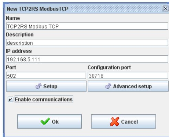
Figure 43: New TCP2RS Modbus TCP
