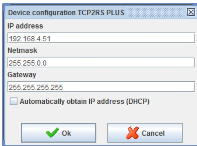
Figure 45: Device configuration TCP2RSPLUS
