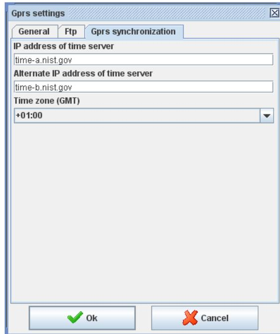
Figure 99:GPRS configuration, GPRS synchronisation
