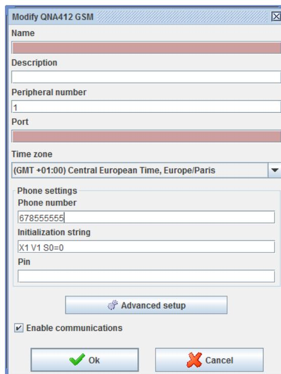
Figure 90: Dialogue box for configuration of QNA412 GSM communications
