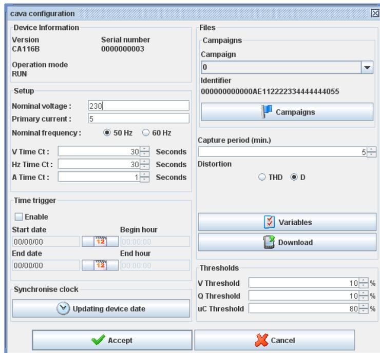
Figure 67: Dialogue box for CAVA device parameter configuration
