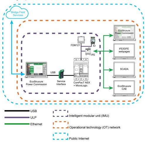
The intelligent modular unit (IMU) represents the ComPacT NSX or PowerPacT H-, J- or L-Frame circuit breaker, the MicroLogic trip unit, and the associated ULP modules, communication interface, and IO modules.
