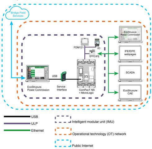
The intelligent modular unit (IMU) represents the MasterPact NT/NW, ComPacT NS, or PowerPacT P- or R-frame circuit breaker, the MicroLogic trip unit, and the associated ULP modules, communication interface, and IO modules.
