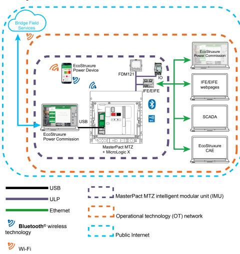
The MasterPact MTZ intelligent modular unit (IMU) represents the circuit breaker, the MicroLogic X control unit, and the associated ULP modules, communication interface, and IO modules.
