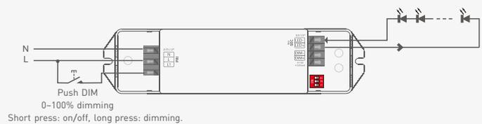
The dimming interface priority: First 0-10V, next Push DIM.
