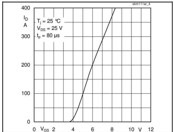
Fig. 4 Transfer characteristic
