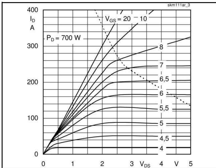
Fig. 3 Output characteristic
