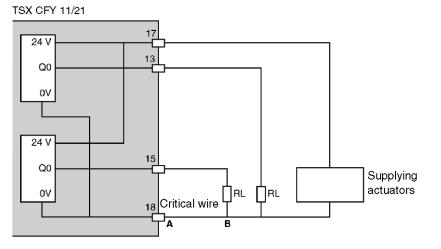
If there is a break of the supply section between A and B, there is a risk that the RL actuators may not remain operational. You must, if possible, double connections of 0 V supply to the modules.
