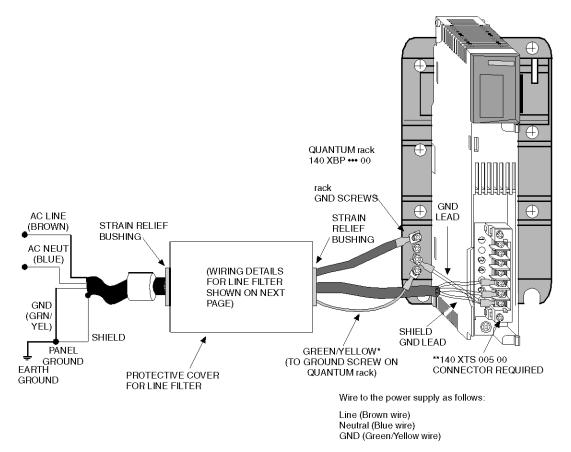
\* Only one ground wire per rack is required. In redundant and summable systems, this lead is not connected for the additional line filter/power supply
