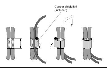
NOTE: The by-pass for the bus ends is to be prepared on **one** cable only
