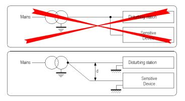
Separate power supplies must be provided if extremely sensitive and high interference devices are used concurrently in the same power supply system:
