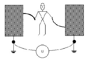
Equipments and electronic systems are interconnected. The best way to ensure that everything works properly is to maintain good equipotentiality between equipments. Besides the safety of the personnel, which is a LF (Low Frequency) constraint, equipotentiality between equipments must be satisfactory, especially for digital equipments even at very high frequencies.
