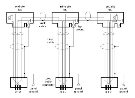
The diagram shows a drop cable, connected and grounded with a tap.
