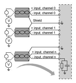
If the sensors are referenced in relation to the ground, this may in some cases return a remote ground potential to the terminal or the Sub-D connector(s). It is therefore necessary to follow the following rules:
