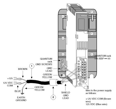
**NOTE:** For detailed wiring diagrams of power supply modules, refer to the part Part Power Supplies (see *Quantum using EcoStruxure*<sup>™</sup> *Control Expert, Hardware, Reference Manual*).
