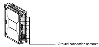
Precautions to be taken when replacing a PCX 57 processor
