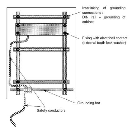
**NOTE:** All the fixing must be with an electrical contact. You have to scrape the paint.
