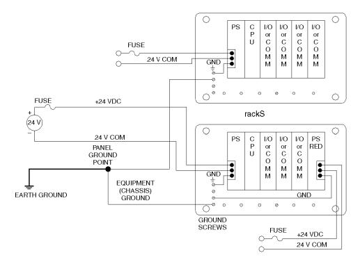
NOTE: It is recommended to earth ground the 24 VDC power supply.
