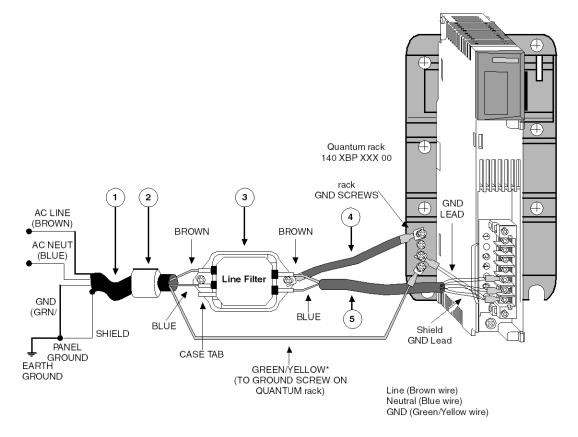
**NOTE:** Only one ground wire per rack is required. In redundant and summable systems, this lead is not connected for the additional line filter/power supply.
