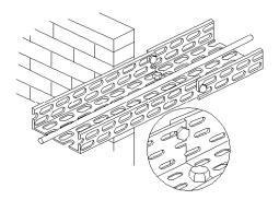
**NOTE:** The earthing of cable ducts must be carried out when necessary, see Direct bonding by bolted fastening for metallic parts, page 90.
