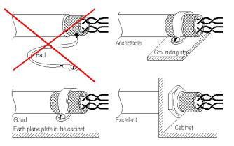
**NOTE:** The ground connection for cable shields must always run through the entire cable.
