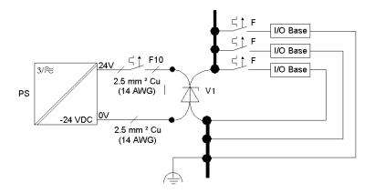
**F** automatic circuit breaker or fuse (see appropriate field wiring illustration in I/O base description)
