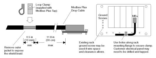
**NOTE:** To maintain CE compliance with the European Directive on EMC (89/336/EEC), the Modbus Plus drop cables must be installed in accordance with these instructions.
