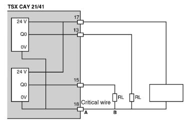
If there is a break of the supply section between A and B, there is a risk that the RL actuators may not remain operational. You must, if possible, double connections of 0 V supply to the modules.
