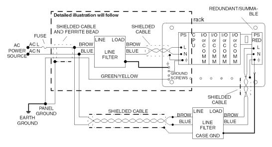
**NOTE:** To maintain CE compliance with the European Directive on EMC (89/336/EEC), the AC power supplies must be installed per the European Directive on EMC (89/336/EEC).
