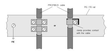
**NOTE:** An equalization current can flow across a shield connected at both ends because of fluctuations in ground potential. To prevent this, it is imperative that there is potential equalization between all the attached installation components and devices.
