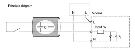
• the line capacity values that must not be exceeded are given in the summary table at the end of this paragraph.
