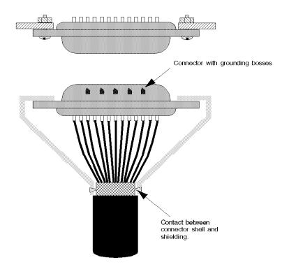
The graph below shows the right way to build a connector-type connection:
