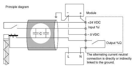
When the input contact is open, an alternating current exceeding the cable's interference capacities may generate a current in the input which might cause it to be set to 1.
