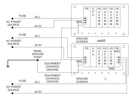
**NOTE:** \*AC N should be earth grounded. If it is not earth grounded, it must be fused (refer to local codes).
