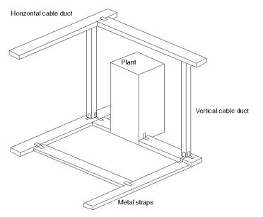
**NOTE:** Sensor and actuator cables **outside of** these islands must be shielded with great care!
