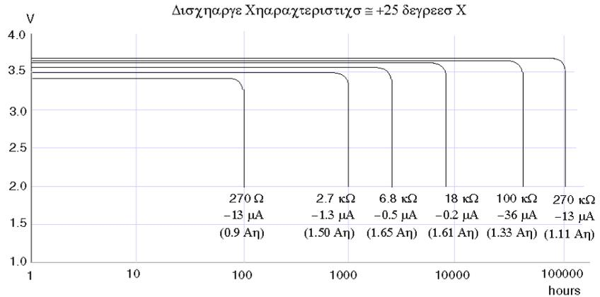
At higher temperatures, alkaline aging accelerates well ahead of lithium. The 3.6 V rating of this lithium battery is well above the 2.68 V battery-low threshold, further supporting the improved and extended service life over the AAA alkalines.
