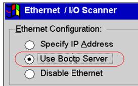
If the processor adapter is powered up without battery backup, and its IP address was previously saved to flash, the adapter will issue three BOOTP requests five seconds apart.
