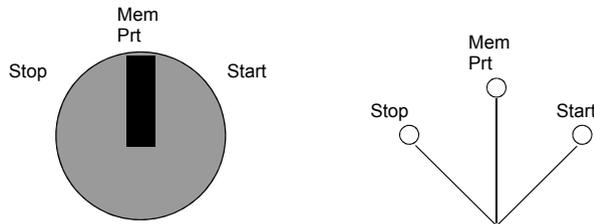
**Note:** The key switch positions shown next to the switch (above) are for reference only and are marked on the module as indicated on the right.
