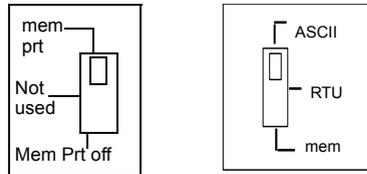
**Note:** The CPU hardware defaults to bridge mode when the front panel switch is set to RTU or ASCII mode. When networking controllers, a panel device connected to the CPU Modbus port can communicate with the controller to which it is connected, as well as log into any nodes on the Modbus Plus network.
