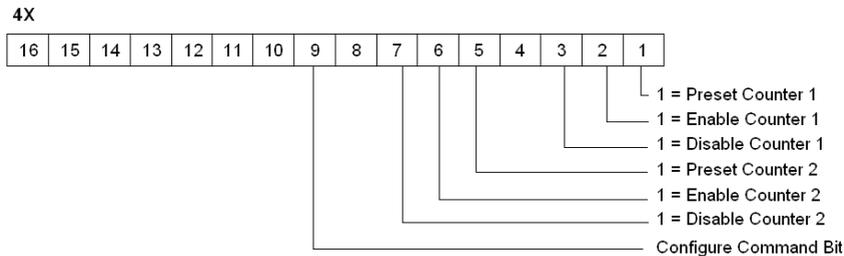
The following figure shows the 4x + 1 output register for command 1 (4X+1).
