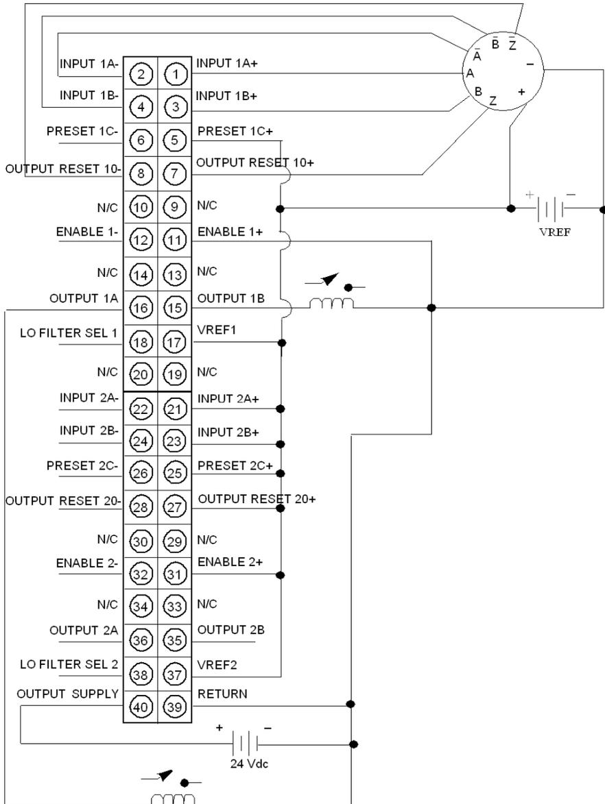
**NOTE:** Zero pulse resets Output 1A and 1B
