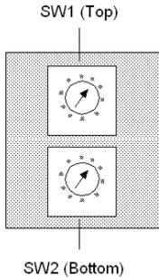
**NOTE:** If "0," or an address greater than 64 is selected, the Modbus + LED will be "on" steady, to indicate the selection of an invalid address.
