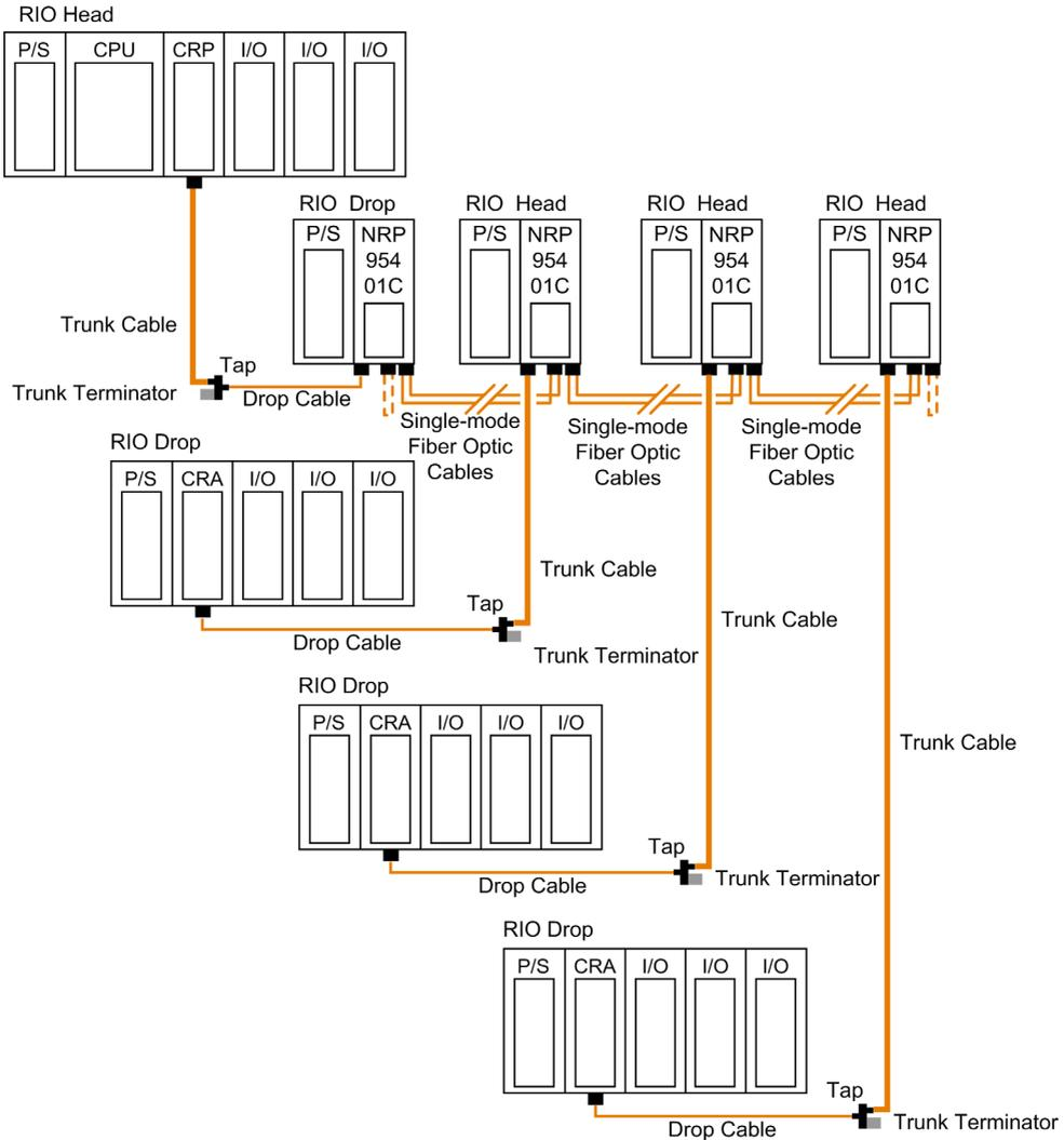
**NOTE:** The total distance between the first and the last fiber optic repeater is limited by the maximum allowable power loss from end-to-end (16 km over 9/125 μm fiber). Power loss includes the fiber optic cable attenuation, connector losses at the fiber optic receiver and transmitter ports, and the system margin of 3 dB.
