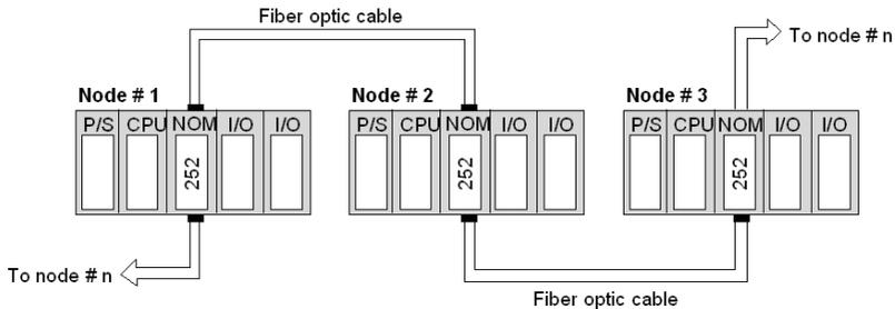
**NOTE:** The distance between nodes on fiber is limited by the maximum allowable power loss from end-to-end (3 km over 62.5 mm fiber). Power loss includes the fiber optic cable attenuation, connector losses at the Fiber Optic Receiver and Transmitter ports, and the system margin of 3 dB. In this configuration, the end NOM 252 00 in this configuration will have the FRNGoff LED active. It also displays the Cable B Framing error in the MBPSTAT (in ladder logic).
