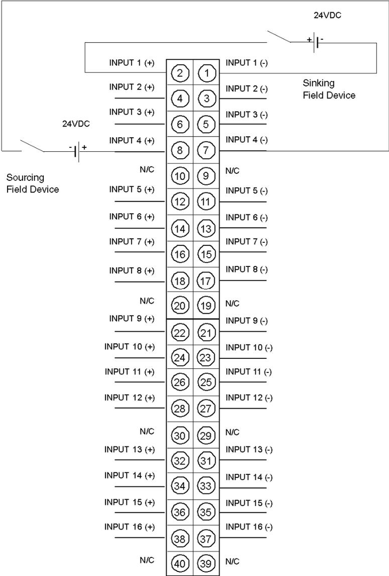
**NOTE:** Either shielded or unshielded signal cables may be used (the user should consider using shielded wire in a noisy environment). Shielded types should have a shield tied to earth ground near the signal ground.
