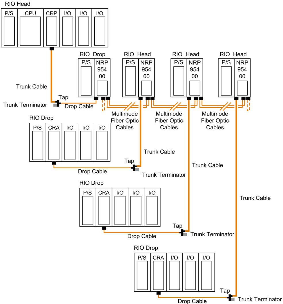
**NOTE:** The distance between nodes on fiber is limited by the maximum allowable power loss from end-to-end (3 km over 62.5 μm fiber). Power loss includes the fiber optic cable attenuation, connector losses at the fiber optic receiver and transmitter ports, and the system margin of 3 dB.
