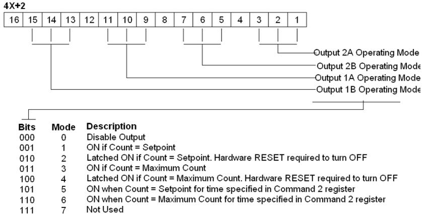
**NOTE:** The Output ON time specified in the Command 2 registers may be used by only one of the four outputs. When more than one output is set to mode 5 or 6, the module firmware will operate the first one encountered, and disable the other outputs set to modes 5 or 6.
