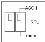
**NOTE:** If the left-hand switch is in the upper position and right-hand switch is set to mem then, as of firmware version 2.20, bridge mode is deactivated. This means that the network connection between Modbus and Modbus Plus is locked.
