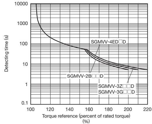
Note: Overload characteristics shown above do not guarantee continuous duty of 100% or more output.
