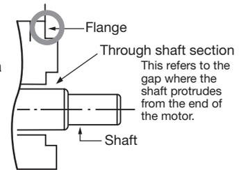
Precautions on Using Servomotor with Oil Seal:
