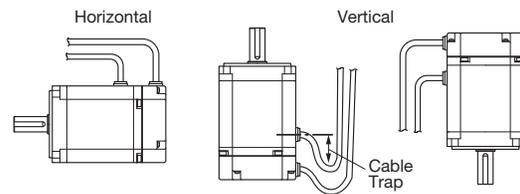
Note: When installing servomotors vertically, make cable traps to keep out water. When mounting servomotors with the shaft up, take measures with the connected machine to prevent oil from getting into the servomotors through gear boxes etc.
