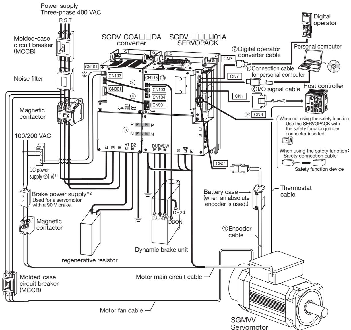
\*1 : You must provide the 24-VDC power supply. Use a 24-VDC power supply with double insulation or reinforced insulation.
