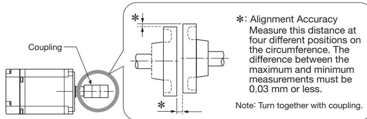
2 Do not allow any direct impact to the shafts when installing the couplings. Do not hit the area near encoders with a hammer etc., as impacts may damage the encoders.
