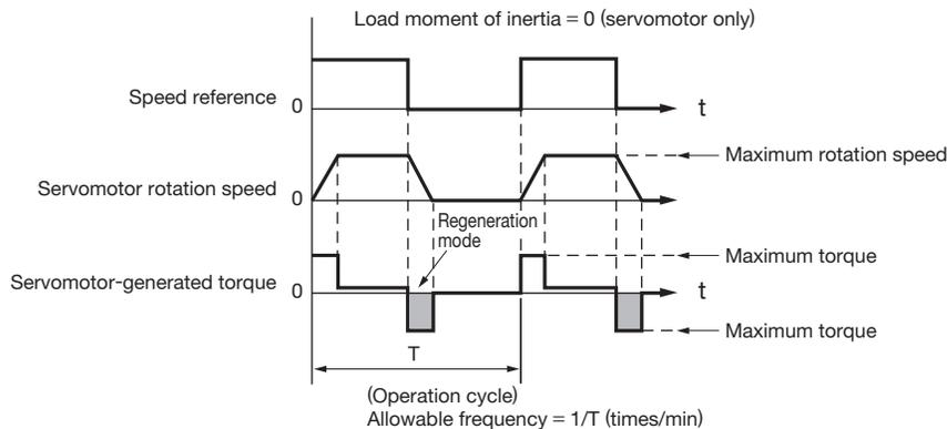
Use the following equation to calculate the allowable frequency for regeneration mode operation
