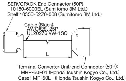
Note: The pin numbers in the SERVOPACK connector and the pin numbers in the terminal block are the same. If assembling cables, refer to **●Cable with Loose Wires at One End for CN1 Connection Diagram of JZSP-CVI01-□-E Cable** on the next page.
