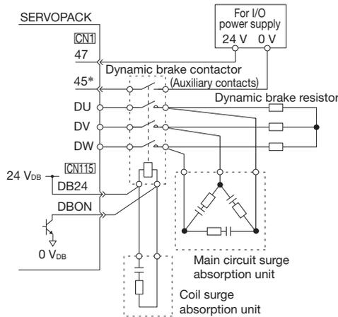
\*: The above figure is for using a dynamic brake contactor with NO contacts. The dynamic brake answer signal (a signal from NO auxiliary contacts) is input to CN1-45. To indicate an error if the input signal to CN1-45 turns OFF (open) while the dynamic brake is activated, the Pn515 parameter in the SERVOPACK must be set to n.□E□□. If the dynamic brake answer signal is not used, Pn515 is set to n.□8□□ (default setting).
