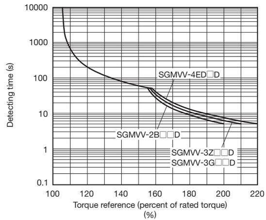
Note: Overload characteristics shown above do not guarantee continuous duty of 100% or more output. Use a servomotor with effective torque within the continuous duty zone of *Torque-Motor Speed Characteristics*.
