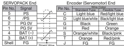
Note: The signals BAT (+) and BAT (-) are used when using an absolute encoder.
