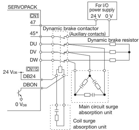
\*: The above figure is for using a dynamic brake contactor with NC contacts. The dynamic brake answer signal (a signal from NC auxiliary contacts) is input to CN1-45. To indicate an error if the input signal to CN1-45 turns OFF (open) while the dynamic brake is activated, the Pn515 parameter in the SERVOPACK must be set to n.□E□□. If the dynamic brake answer signal is not used, Pn515 is set to n.□8□□ (default setting).
