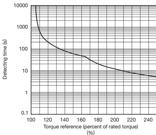
Motors with Rated Speed of 800 RPM
