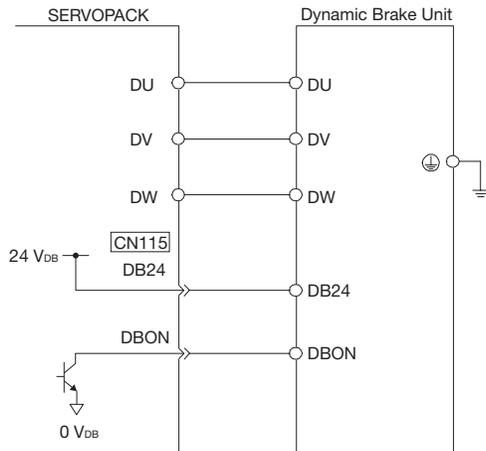
Note: The dynamic brake answer function cannot be used because there are no auxiliary contacts on the contactor.
