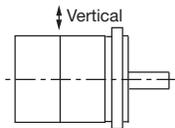
Impact Applied to the Servomotor
