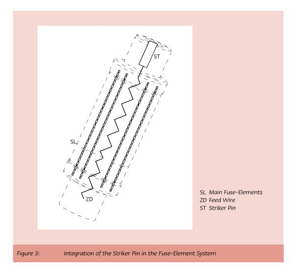
Alongside the fuse housing with its contact caps and the fuse-elements, the striker pin is thus another essential constituent of a high-voltage fuse. The overall system consists of the striker pin which is visible for the user and red in most cases, a coil spring providing the tripping energy, a holding wire retaining the spring and a feed wire for contacting the tripping system. Figure 2 shows a striker pin structured that way.
