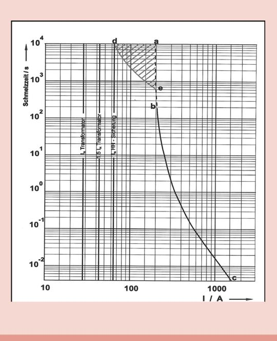
Figure 6: Time-Current Characteristic of a 63 A HV Fuse with a Temperature Limiting Striker Pin in relation to the Operating Currents of a 1 000 kVA Transformer
