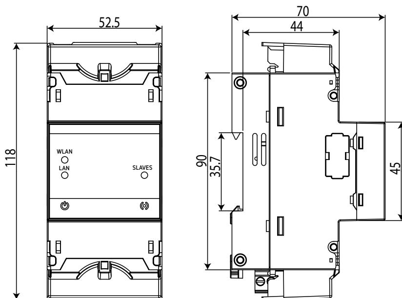
Figure 45: line-EDS-Cloud dimensions.
