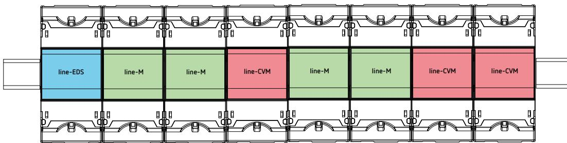
Figure 5: Typical installation of a line-EDS-Cloud with 7 devices.
