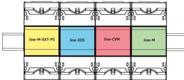
Figure 6: Maximum set a line-M-EXT-PS can supply.
