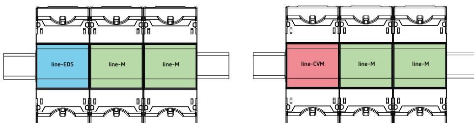
Figure 4: line-EDS-Cloud and line CVM expansion module connection.
