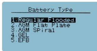
2.Select the battery type (Support regular flooded / GEL / AGM / EFB)
