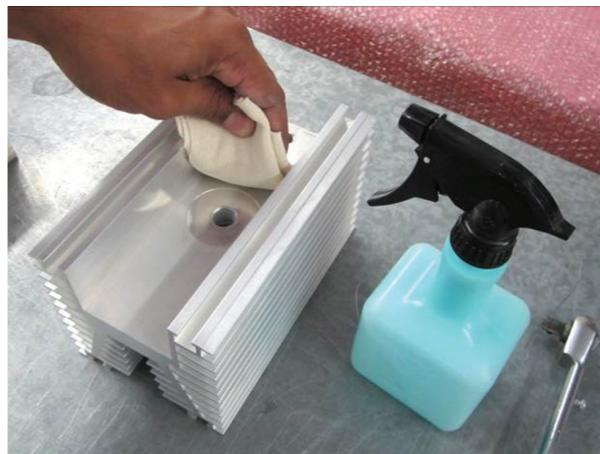
**1<sup>st</sup> Step:** Clean up the heatsink or metal plate with isopropyl alcohol. The fixing hole should be cleaned as well to remove oil, greases and other chemical residues.
