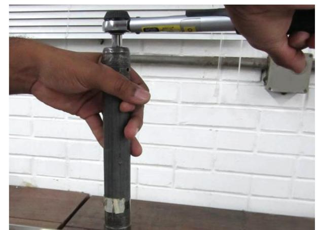
**4<sup>th</sup> Step:** Apply the datasheet recommended torque in the device with a properly adjusted torque wrench. It is very important stop torqueing when the signal that adjusted torque was reached is emitted. The click-type will emit a click sound and the break-over type will deflect its handle. Tightening must be stopped, to avoid excessive torque over the device.
