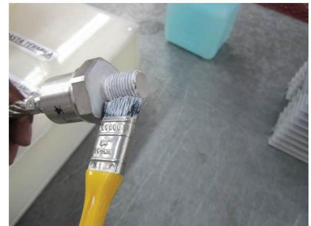
**2<sup>nd</sup> Step:** Apply a thin layer of thermal paste (60 µm maximum) with the brush. SEMIKRON indicates Wacker P12 thermal paste to mount stud type devices.
