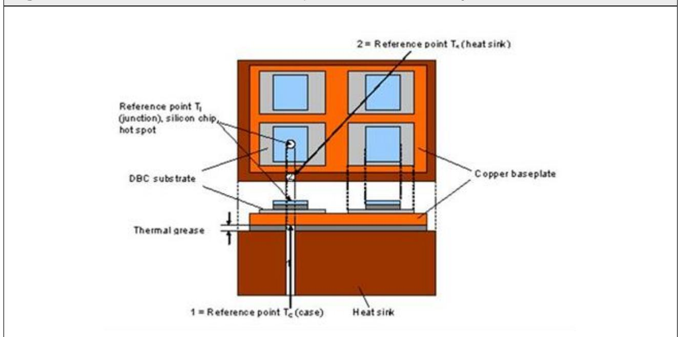
**Figure 7: Method B, location of reference points for Rth measurement**
