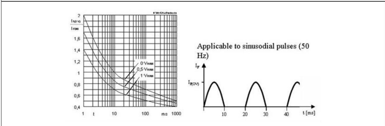
Peak value of overload current  $I_{T(OV)}$  permissible under fault conditions normalised to the surge on-state current  $I_{TSM}$  shown as a function of the duration of the fault  $t$ . The parameter is the peak reverse voltage to be reapplied immediately after the fault current has ceased. For faults lasting longer than 10 ms the graph assumes the current waveform to be a series of half sinewaves of 8.3 or 10 ms duration occurring at a rate of one every 16.6 or 20 ms.
