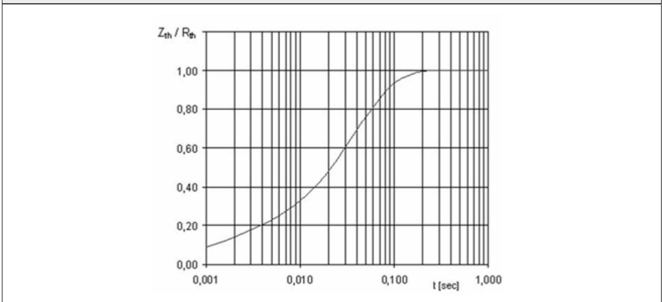
During SEMIKRON’s module qualification process the transient thermal behaviour is measured. On the basis of this measurement mathematical model is derived, resulting in the following equation (3-2):
