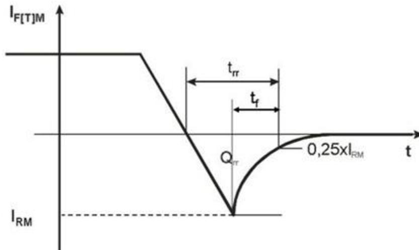
The following relations exist between  $t_{rr}$ ,  $Q_{rr}$ , the current fall time  $t_f$  and the peak reverse recovery current  $I_{RM}$  (cf. Fig. 1 of the datasheet):
