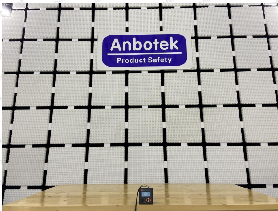
Photo of RF Field Strength susceptibility Test
