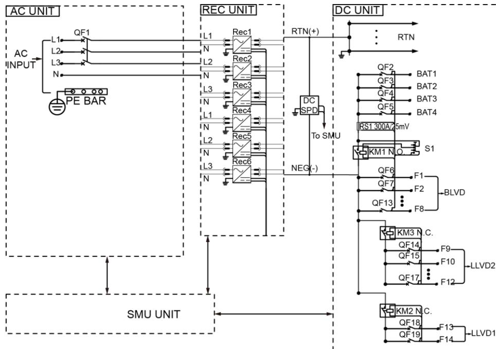
Figure B-2 DCDB electrical conceptual diagram
