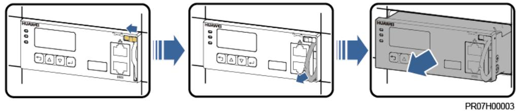
**Step 3** Insert the new SMU into the subrack, push the locking latch towards the left, and pull out the handle.
