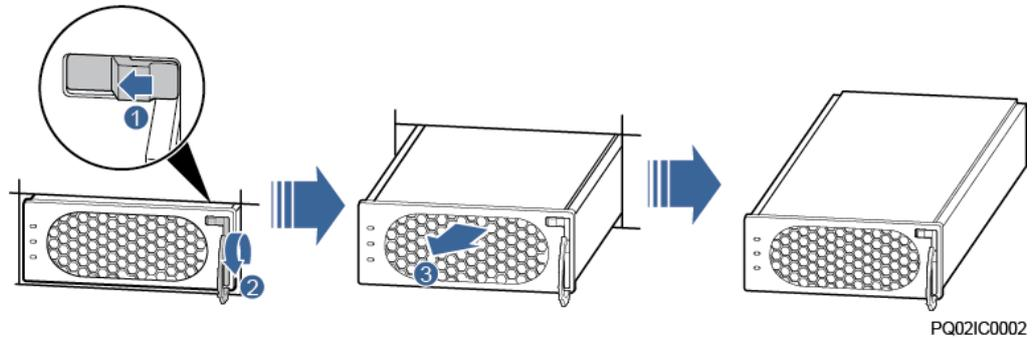
**Step 4** Push the locking latch on the new rectifier towards the left, and pull out the handle.
