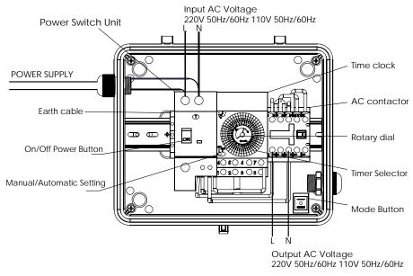
⚠ Warning: Maximum load of the Control Box must not exceed 2.2KW.
