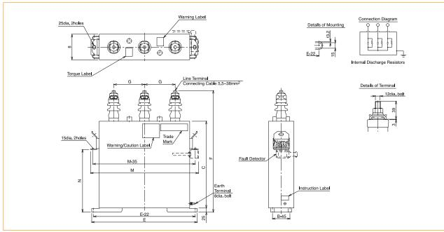
(Notes) 1. To assemble two or more capacitors, secure the spacing of 80mm or more between the units for the combined output of 150-300kvar and 100mm or more for 400-
